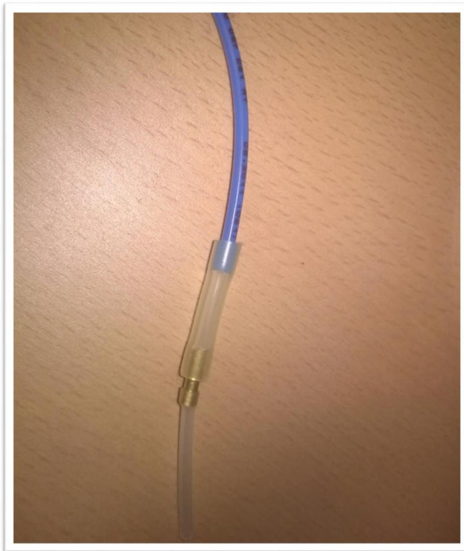
*Figure 10: Example triple transition joint, from 2mm OD silicon tube to brass 3mm OD tube, then to 4mm OD silicone tube and 3mm OD rigid plastic tube. Consider using cable ties to secure the joints.*
