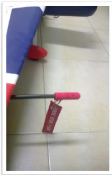
*Figure 2: 8 mm Pitot tube on a commercial air frame*
