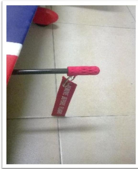
*Figure 13: A Cover for an airspeed probe*
