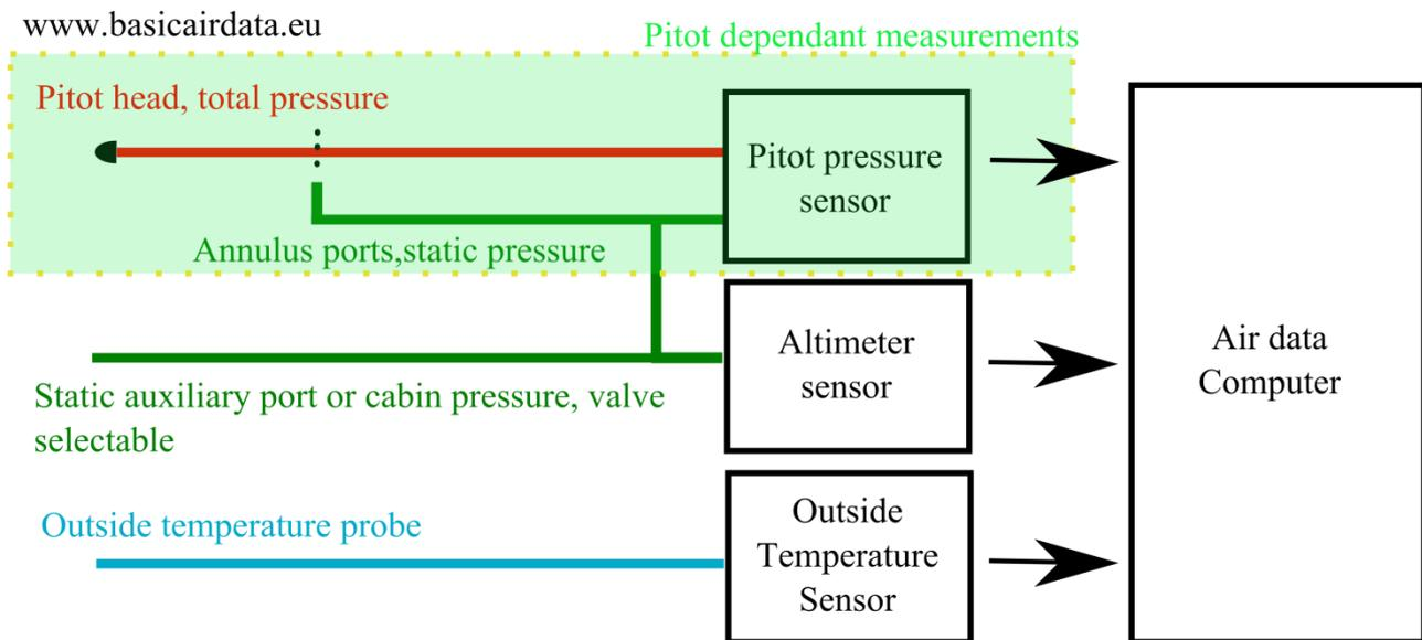
*Figure 14: Air data instruments integration scheme*
