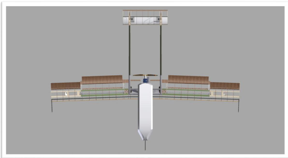
*Figure 1: Air frame equipped with three airspeed probes, on the nosecone and the wingtips*
