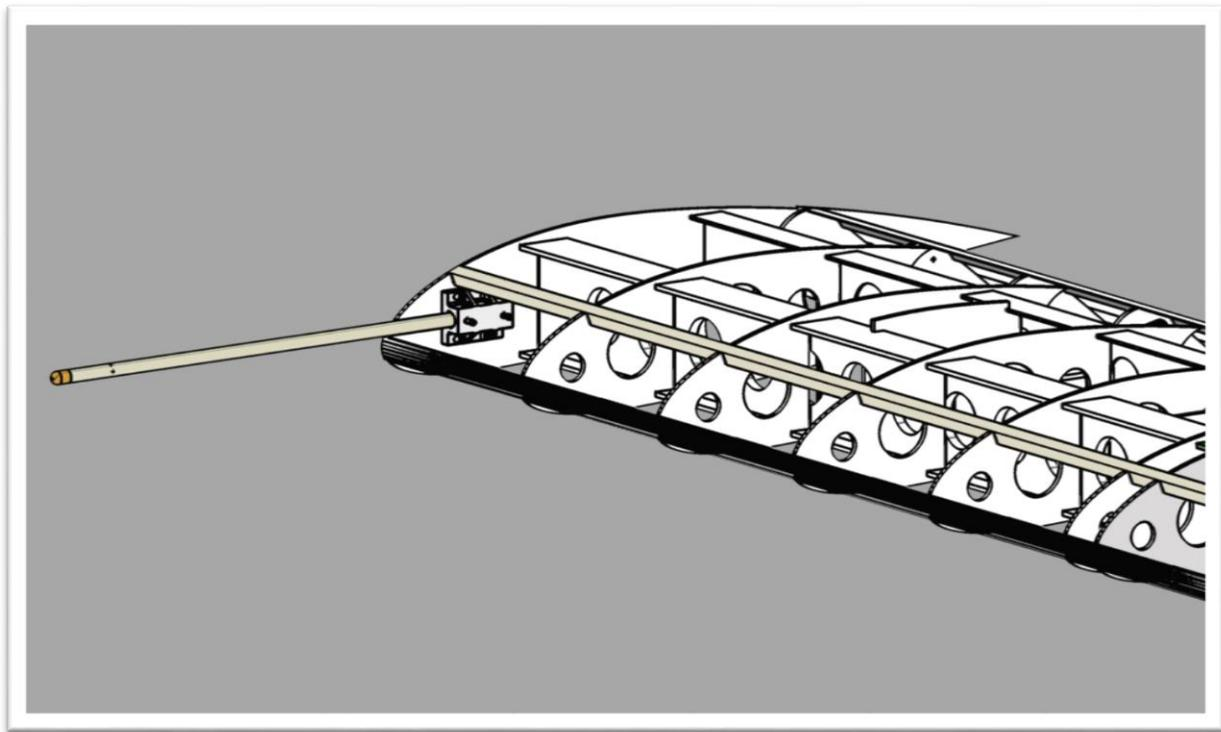
*Figure 3: Wing tip installation, with barbed ports inside the wing*
