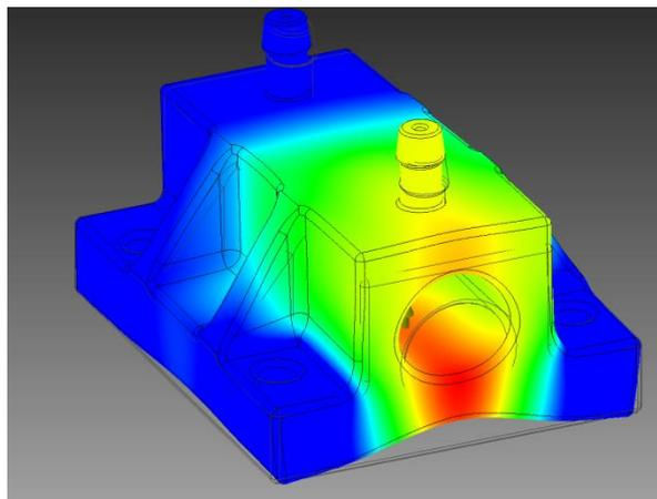
*Figure 16: Flange FEM, maximum deformation in red*
