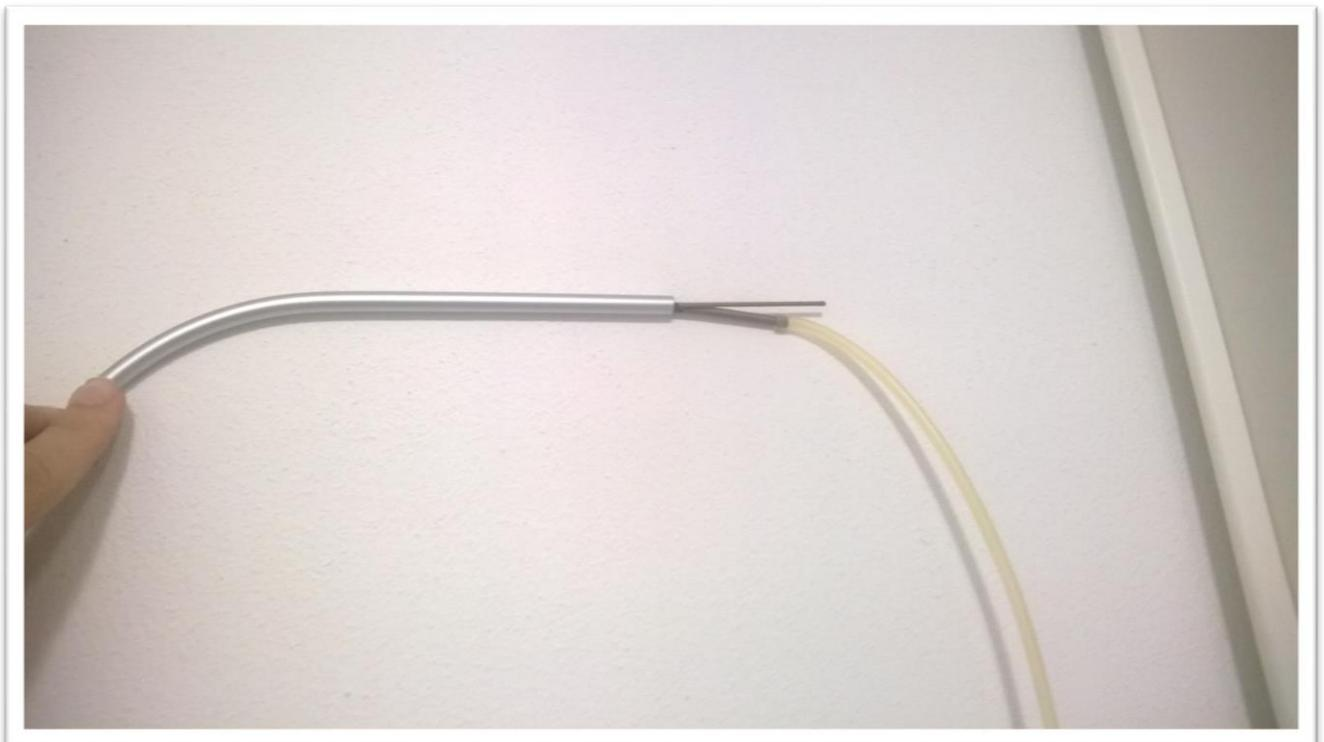
*Figure 9: Pressure tapping on a non-flanged, L-Shaped pitot*
